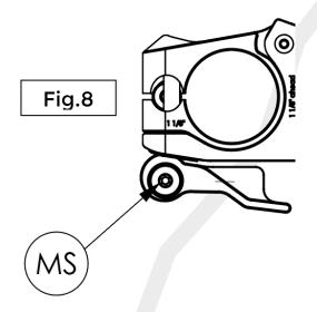
Please loosen the grub screw [MS] in the clamping lever and the counter screw [KS]. Now the clamping screw [SS] can be readjusted slightly (see description in FIG. 7). Now the grub screw and the counter screw must be tightened hand-tight again.
