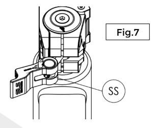
If the tensioning lever **[SH]** becomes loose over time due to frequent use, it is possible to secure it against twisting again.
