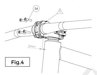
The handlebar covers must be attached to the stem using the top two clamping screws [S4] [Fig. 4]. After aligning the handlebars in height and inclination, tighten the screws [S4] [Fig.4] with a torque of 8Nm (first the top two screws, then the bottom two screws!).
