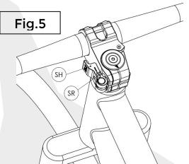
stem/handlebar The can now be swiveled 90° to the side. This locks into the end position. In this position, please do not lift the bike by the handlebars!
