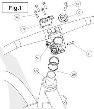
The stem must be aligned using spacer rings [DR] (accessory, not included) so that it protrudes approx. 1.5 - 2 mm above the fork shaft. After aligning, adjust the bearing play by tightening the ahead cover [D] with the screw [S3] with approx. 1.5 - 2 Nm. Make sure that the clamping screw [S1] is loose.
