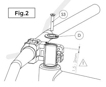
When closed (not swiveled), the stem must be aligned so that it is transverse to the direction of travel. First tighten the clamping screw [S1] hand-tight. Then open the swivel mechanism, insert the clamping screw [S2] and tighten the clamping screws [S1] and [S2] with a torque of 6Nm.
