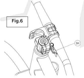
The stem/handlebar can now be swiveled 90° to the side. This engages in the end position. Please tighten the clamping lever [SH] in the "park position" [Fig. 6]. Do not lift the bike by the handlebars in this position!
