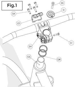
Align the stem using spacer rings [DR] (accessory, not included) so that it protrudes approx. 1.5 - 2 mm above the steerer tube. After alignment, adjust the bearing play by tightening the Ahead cap [D] with the bolt [S3] to approx. 1.5 - 2 Nm. Make sure that the clamping screw [S1] is loose.
