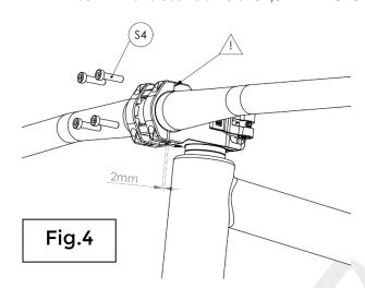
To swivel the stem, push the locking bolt [SR] forwards. Only then can the clamping lever [SH] be opened.
