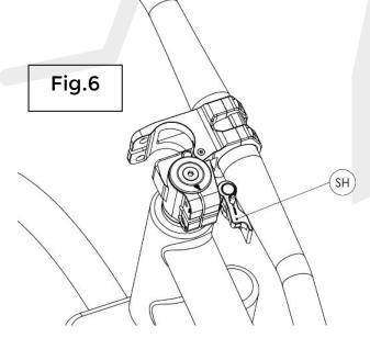
The stem/handlebar can now be swiveled 90° to the side. This engages in the end position. Please tighten the clamping lever [SH] in the "park position" [Fig. 6]. Do not lift the bike by the handlebars in this position!
