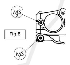
If the clamping lever [SH] becomes slightly loose over time due to frequent adjustment of the pre-tensioning force [FIG.7], it can be secured again from below with the two grub screws [MS1 and MS2]. Please note that the lower clamping screw [S2] must be removed for this and tightened again with a torque of 6 Nm after screwing it in.
