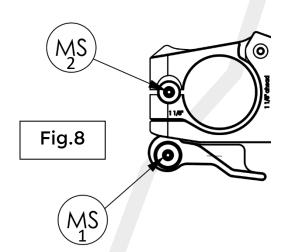
If the clamping lever [SH] becomes slightly loose over time due to frequent adjustment of the pre-tensioning force [FIG.7], it can be secured again from below with the two grub screws [MS1 and MS2]. Please note that the lower clamping screw [S2] must be removed for this and tightened again with a torque of 6 Nm after screwing it in.
